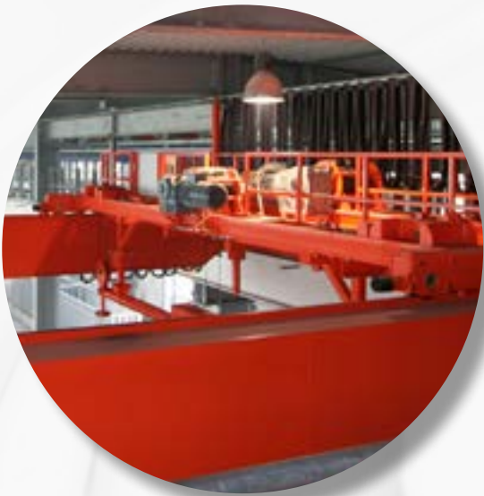
1. The crane trolley in the galvanizing plant receives and sends data via DATAEAGLE slave.
