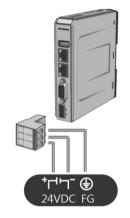
NOTE: Connect positive DC line to the '+' terminal and the DC ground to the '-' terminal.
